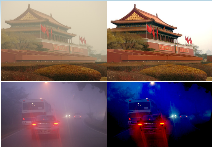
Figure: Daytime dehazing method of Fattal[1] failing for night time images. Include miri haze here
